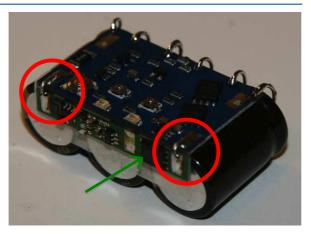
2. Solder cables as shown below. The ground (-) from both the BEC and MP-GCG1 output are now common and must be soldered to the left most solder point. The positive (+) lead from the BEC is soldered to the middle solder point. The positive lead (+) to the RC systems is soldered to the right solder point.
