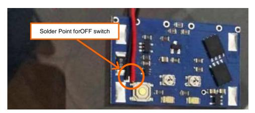
2. The external "ON" switch is installed between the positive (+) LiPo and positive (+) output solder points as depicted below:
