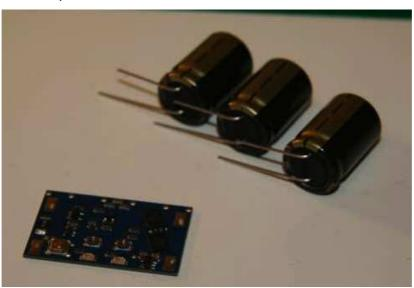
2. Insertcapacitors into circuit board as in the picture below
