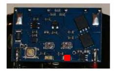
The unit automatically begins charging the capacitors (NC) or LiPo (NL). ). When the charge reaches 85% the green LED lights.
